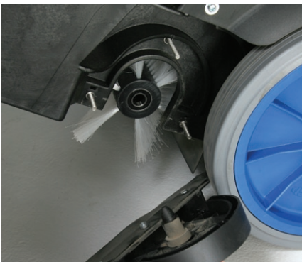
No tools required for changing, inspecting or adjusting the main broom.
